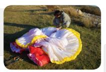
Step 2. Group leading edge (LE) plastic reinforcements with the A tabs roughly aligned. Make sure the plastic reinforcements lay side by side. Note the glider is NOT folded in half; it is folded as a complete concertina from wing tip to wing tip.
