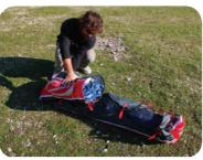
IMPORTANT: Do NOT lay the wing flat on the ground before packing the glider, this will cause abrasion damage to the top surface as you pull the glider towards the middle. ALWAYS pack from a mushroom or lift the wing off the ground when gathering the wing and grouping the leading edge.
