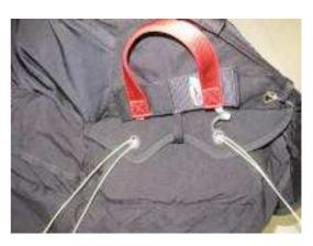
Then the packing cords are threaded through the eyelets of the upper flap.
