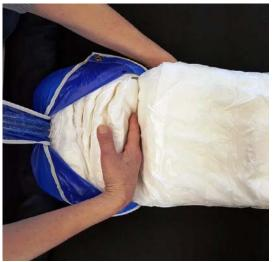
Now put the canopy into the inner container. Close both sides of the inner container with the white rubber band and pull the suspension lines through the rubber band for closing.
