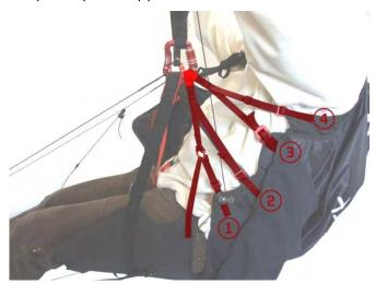
In the detail photo, adjustment n° 1 changes the angle between thighs and back (seat depth), distributing load between seat and the lumbar area and thus improving pilot comfort.
