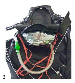
The ballast lodging is located beneath the seat. Open the zipper to access (1) the lodging, insert the discharge tube into the through-hole on the right (2) and install the ballast (3).
