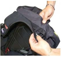
The two connections should be made using screw-lock karabiners with a breaking strength of at least 1,400 kg. In any case, it is important to verify that the length of the bridle is sufficient to position the reserve parachute inside the harness pocket, and that there is sufficient play to enable the parachute to be taken out of the pocket without causing the reserve parachute deployment bag itself to open during extraction.
