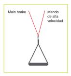
The DOBERMANN 2's high-speed tip is a simple and effective tool. It is a single line from the riser to a critical point of the wingtip. This critical location ensures that, when using the high-speed tip, creases will not appear and the trailing edge or the reflex is not engaged, which might compromise the safety and performance of the wing.
