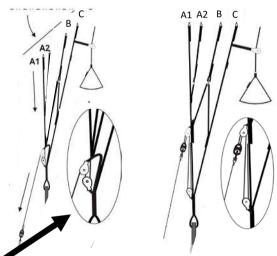
Please pay attention that the glider will not be pre-accelerated, while the accelerator is loosened, when the acceleration ropes are set too short.
