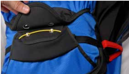
The yellow cable locks the reserve parachute pocket flaps in place. Tuck the upper flap inside its lower stretchable pocket. Check before every flight for the yellow cable to be properly inserted through the two elasticated loops keeping the reserve parachute pocket securely
