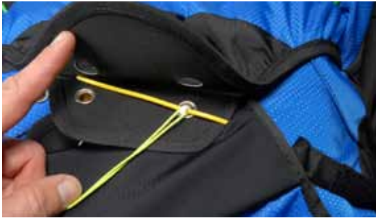
Push the yellow cable through the elasticated loop and gently pull the cord out.
