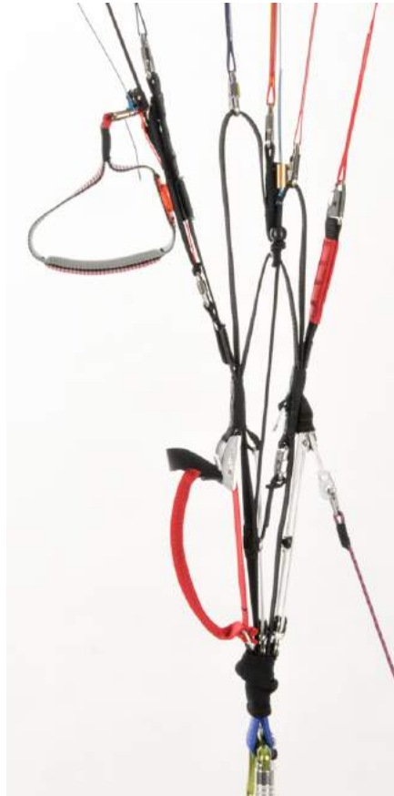
Open trimmers (Fig. 13c) When the trimmers are fully open (the D-riser is lengthened by 100 mm) the reflex
