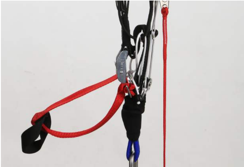
Fig. 11: Overview picture of the riser with the trimmer
