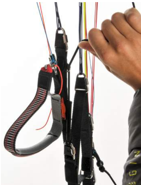
Fig. 18: Wing tip brake with elastic rope and slider on D-riser
