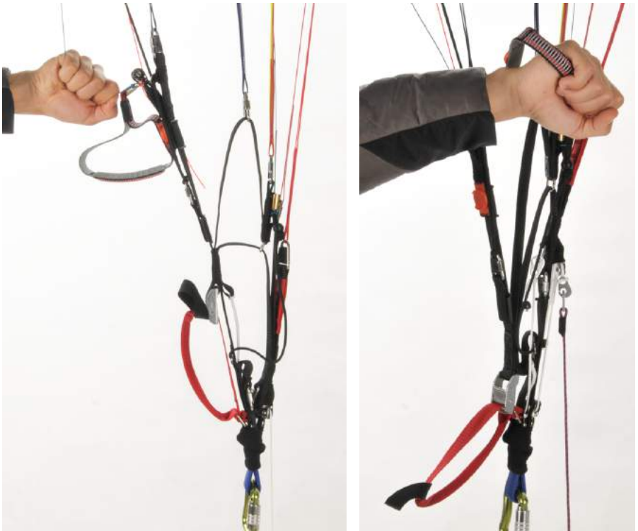
Fig. 4a, b, c, d: Steering with outer 2D steering line only (Trim speed and accelerated)
