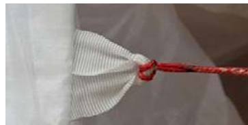
Looped junction - incorrect
