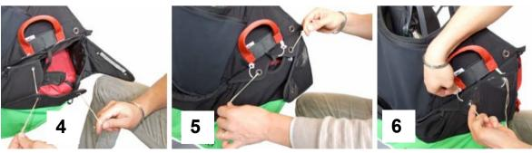
Then begin to close the various parachute container flaps, following the progressive order in the photographs, taking care during this phase that the zip does not open back up at the right end.
