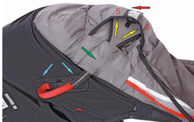
7. Place top of container flap 6 into slot of flap 5 (red arrow). Place release handle underneath flap 5 and 6 (yellow arrows) and cover (green arrow). Close cover and put the handle in the handle slots (blue arrows).
