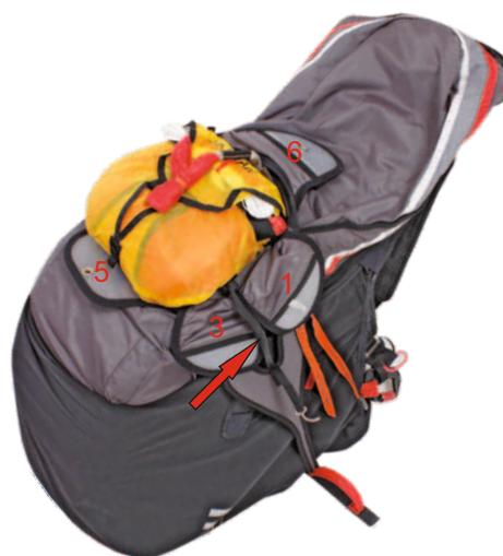
2. Put the deployment bag on the harness container. Stow the bridle in the harness container. The handle connection of the deployment bag leaves in between container flap 1 and 3 (red arrow).
