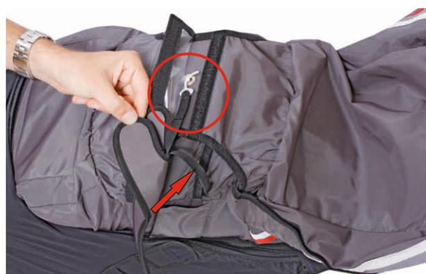
6. Secure the container with the release pin, remove packing needle and packing cord. Close the transparent cover (red circle). Make sure that the connecting band to the rescue system is long enough to release the pin safely (red arrow).
