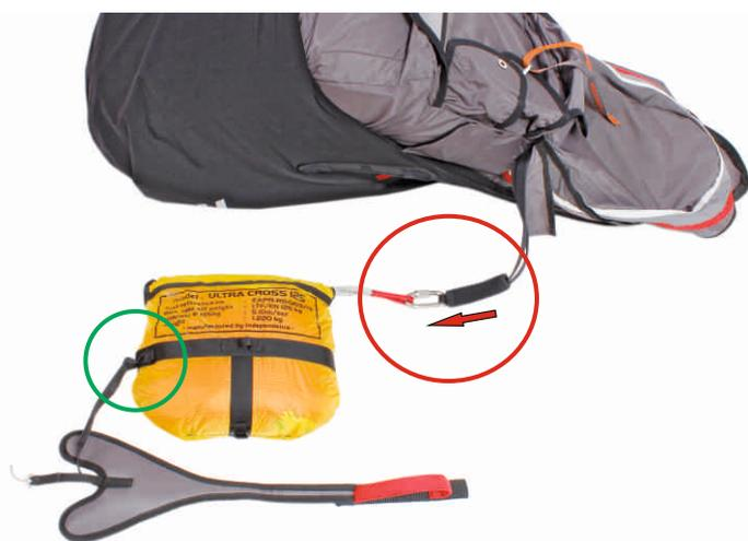
1. Connect the rescue bridle with the harness bridle by looping the bridles or with a quick link (strength > 2400 daN) and fix the connection to prevent slipping (for example by a neopren sleeve as shown in the red circle). Loop in release handle with deployment bag. It is best done if a loop on the side of the deployment bag is used to ensure a reliable release (green circle).
