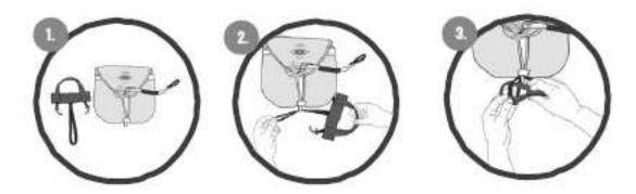
The rescuer handle must be firmly connected to the loop that is attached to the inner container.
