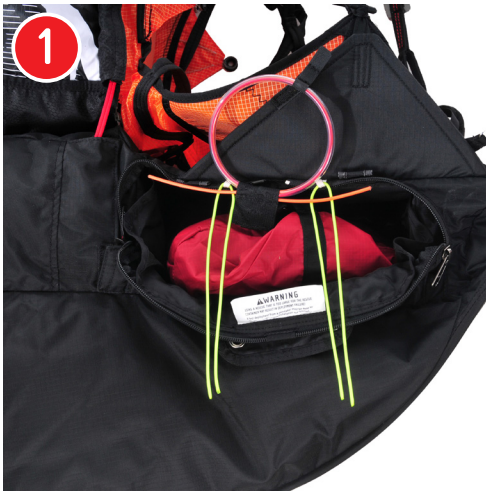
1 Insert reserve with rescue bridle on bottom and handle attachment facing out
