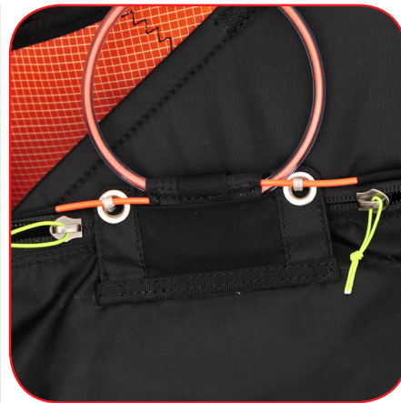
Place the rescue handle into outer cover pocket
