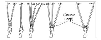
Factory delivered configuration with double loop on C / D-riser lines for trimming during aging
